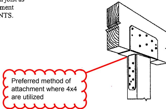
**Figure 11: Rim Joist Connection Details**
