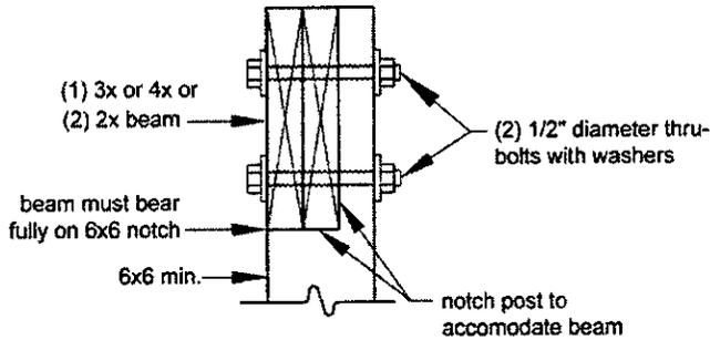
**Figure 9: Prohibited Post-to-Beam Attachment Condition**
