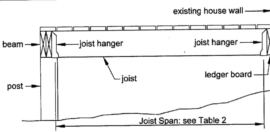
**Figure 2: Joist Span – Free Standing Deck**
