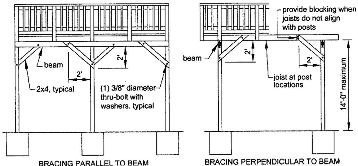
**Diagonal Bracing:** Provide diagonal bracing both parallel and perpendicular to the beam at each post as shown in Figure 22. When parallel to the beam, the bracing shall be bolted to the post at one end and beam at the other. When perpendicular to the beam, the bracing shall be bolted to the post at one end and a joist or blocking between joists at the other. When a joist does not align with the bracing location, provide blocking between the next adjacent joists.
