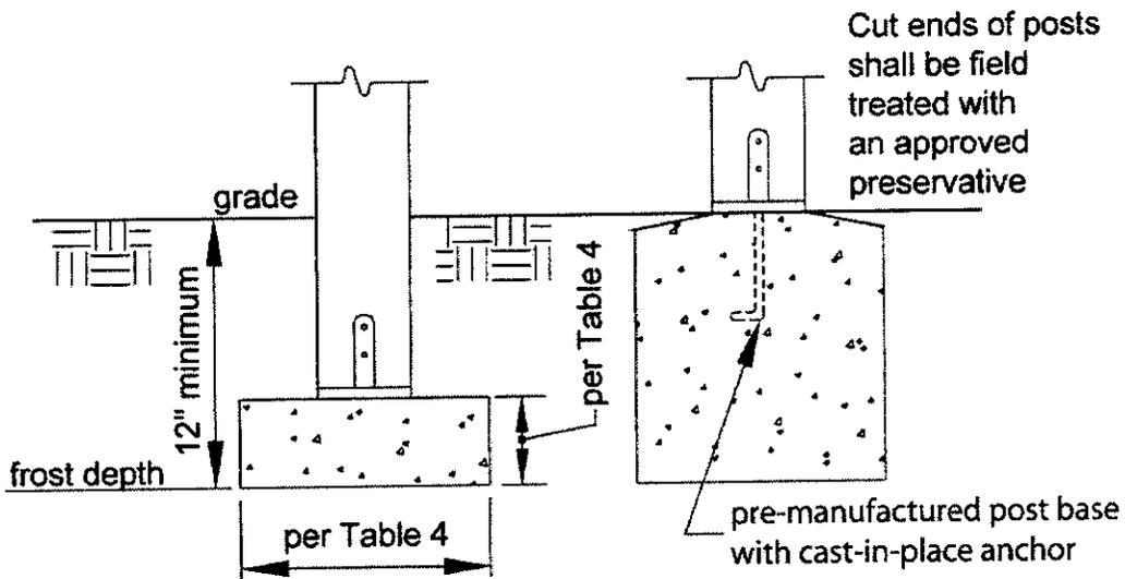
Posts must be anchored to footings. "Embedding" posts directly into footing is acceptable, however, minimum size and thickness of footing may need to be increased to ensure structural integrity of connection
