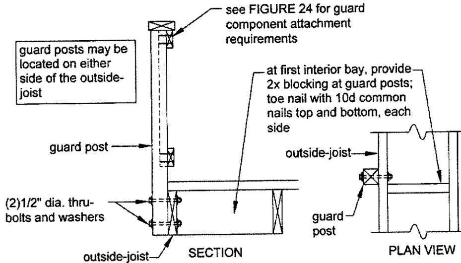
**GUARD POST TO RIM JOIST:** Guard posts for guards that run perpendicular to the deck joists shall be attached to the rim joist in accordance with Figure 26. As shown in Figure 26, hold-down anchors must be installed to attach the guard post and rim joist to the
