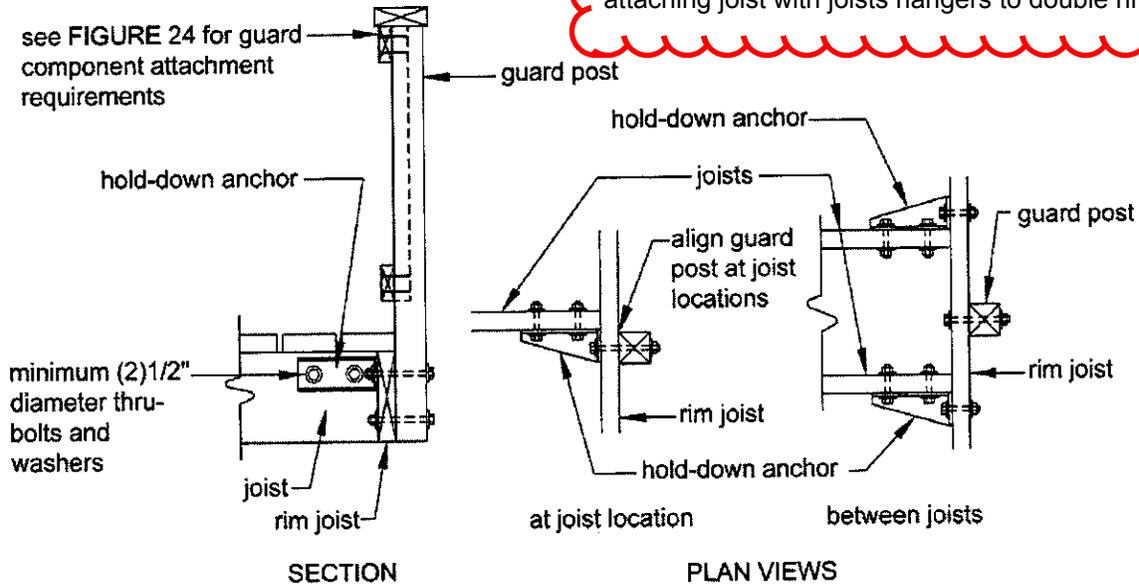
The use of hold down anchors is seen as an option to attaching joist with joists hangers to double rim board
