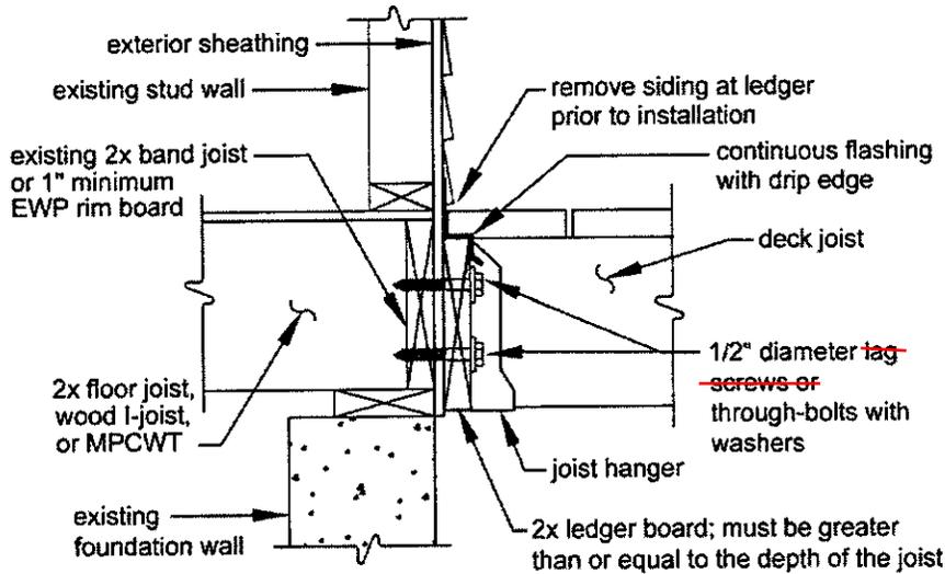
Through bolts, 1/2" diameter spaced in accordance with Table 5.
